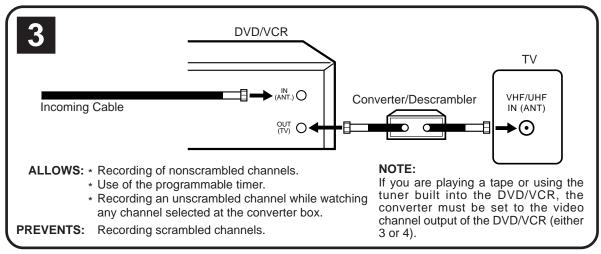
**NOTE:** Whenever a Converter/Descrambler box is placed before the DVD/VCR, you must tune the DVD/VCR to the output of the Converter/Descrambler box, usually channel 3 or 4.
